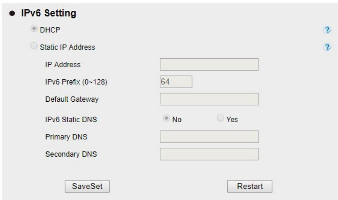
The screenshot shows the 'IPv6 Setting' web interface. It features two radio button options: 'DHCP' (selected) and 'Static IP Address'. Below these are several input fields: 'IP Address', 'IPv6 Prefix (0~128)' (containing '64'), 'Default Gateway', 'IPv6 Static DNS' (with 'No' selected), 'Primary DNS', and 'Secondary DNS'. At the bottom, there are two buttons: 'SaveSet' and 'Restart'. There are also help icons (question marks) next to the radio buttons.
